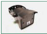
P111407 - FALCON - Universal motion detector which can be installed up to 7 meters. - Vehicle/pedestrian distinction, rejecting parallel traffic. - REMOTE CONTROL programming. - Antenna with planar technology used for the first time in an automatic industrial door, able to provide high precision and stability in the detection field. - IP65
