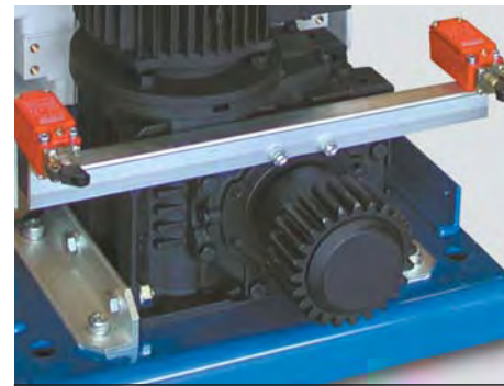
Detail of outer gear and limit switches
