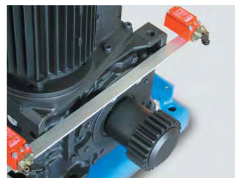
Detail of outer gear and limit switches
